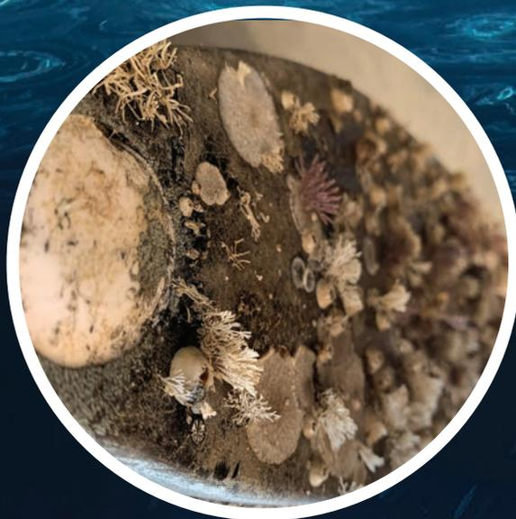
**“As fouling grows on the face of a transducer, the amount of detail that you see is significantly reduced.”**
